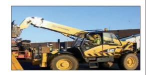
4. The forklift truck operator must position the forks in the most appropriate area to lift the trusses safely. The forklift truck will take the weight of the trusses on the forks.
