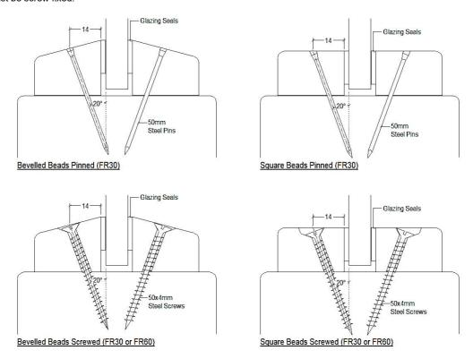
Check the actual thickness of the glass as the manufacturing tolerance can be especially high on the thicker glass types. Fix one set of the beads with the exposed face of the glazing seal off centre in the frame by half the glass thickness. (There are occasions where the glass is installed off centre in the screen, in which case you must follow the contract specific drawings).
