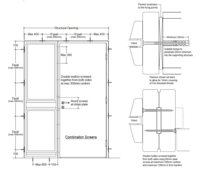
If the screen is part of a doorset combination it is advisable to check the level of the floor screed so that adjustment can be made prior to installation to ensure compliance with threshold gaps, particularly for fire and smoke control. When the installation and finished floor is complete the gap under the door should be no more than 6mm for fire resistance and 3mm for smoke control.
