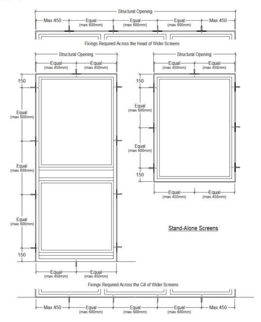
Fixings positions for the jambs should be 150mm from each end and at no more than 600mm centres. At the head and cill the fixings should be at a maximum of 450mm from each end and at no more than 600mm centres.
