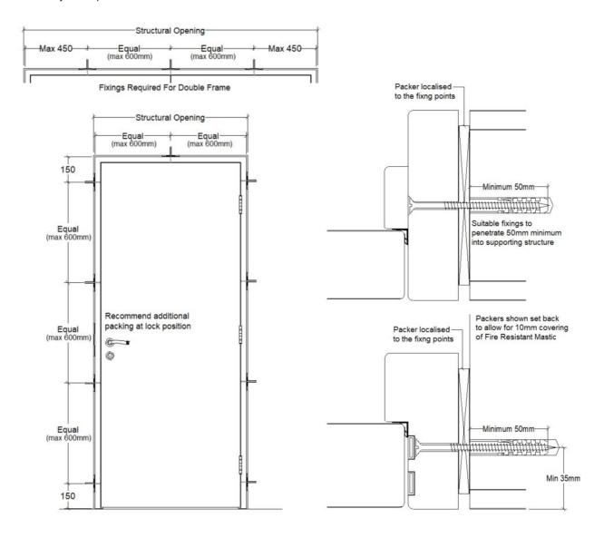
Fixing positions for the jambs should be 150mm from each end and at no more than 600mm centres. For single leaf doorsets less than 1000mm wide it is possible to omit the fixing at the head although we would recommend at least one fixing. For the head of a double frame the fixings should be a maximum 450mm from each end and at no more than 600mm centres. Fixings at the head are used for extra stability and loads that might be imposed by door closers, pivots or other devices.
